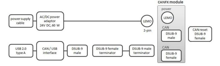
imc CANSAS *flex* capability: built-in terminator resistance, manually switchable
