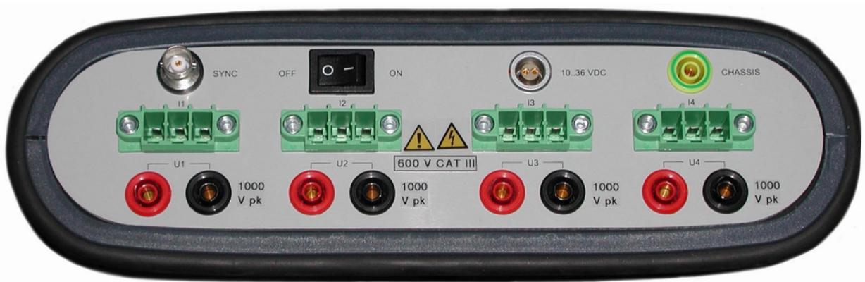
imc POLARES: connection panel for the signals
