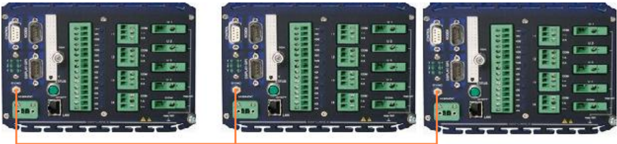
Example for synchronization with master and slave devices
